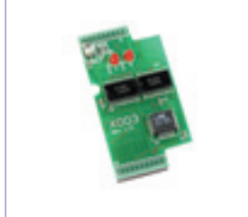
Relay Board X102 (64mm x 32mm)
